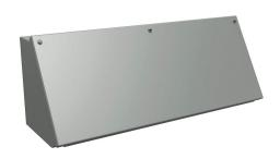
Hammond operator consolet, NEMA 12/13, 7 x 20 x 7in (HxWxD), desktop or pedestal mount, carbon steel, ANSI 61 gray, powder coat finish, screw cover.
