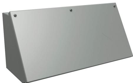
Hammond operator console, NEMA 12/13, 7 x 16 x 7in (HxWxD), desktop or pedestal mount, carbon steel, ANSI 61 gray, powder coat finish, screw cover.
