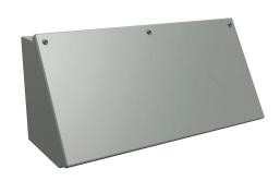
Hammond operator consolet, NEMA 12/13, 7 x 16 x 7in (HxWxD), desktop or pedestal mount, carbon steel, ANSI 61 gray, powder coat finish, screw cover.
