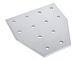
FATH T-shaped flat plate, silver, 12 holes, anodized aluminum, slot size 10. For use with all 45mm and 90mm profile T-slotted rails. Manufacturer part number: 093VT180180D.
