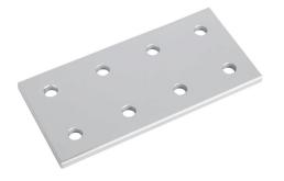
FATH rectangular flat plate, silver, 8 holes, anodized aluminum, slot size 8. For use with all 40mm and 80mm profile T-slotted rails. Manufacturer part number: 093VD80160.
