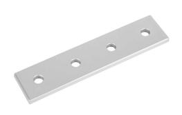
FATH straight flat plate, silver, 4 holes, anodized aluminum, slot size 8. For use with all 40mm and 80mm profile T-slotted rails. Manufacturer part number: 093VA40160.
