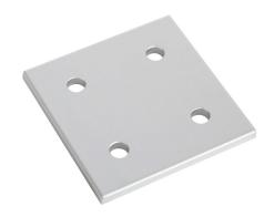
FATH square flat plate, silver, 4 holes, anodized aluminum, slot size 10. For use with all 45mm and 90mm profile T-slotted rails. Manufacturer part number: 093VA9090.
