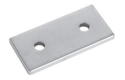
FATH straight flat plate, silver, 2 holes, anodized aluminum, slot size 10. For use with all 45mm and 90mm profile T-slotted rails. Manufacturer part number: 093VA4590.
