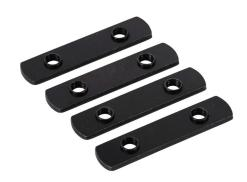
FATH double economy T-nut, black, 5/16-18 UNC, zinc plated steel, slot size 8. Package of 4. For use with all 1.5in and 3in profile T-slotted rails. Manufacturer part number: 096E15U5/16-18S01.
