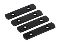
FATH double economy T-nut, black, 5/16-18 UNC, zinc plated steel, slot size 8. Package of 4. For use with all 1.5in and 3in profile T-slotted rails. Manufacturer part number: 096E15U5/16-18S01.
