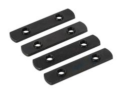
FATH double economy T-nut, black, M8-1.25, zinc plated steel, slot size 8. Package of 4. For use with all 40mm and 80mm profile T-slotted rails. Manufacturer part number: 096E40M8S04.
