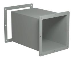
Hammond 1487 series pull-through wireway fitting, cut-off fitting, 8 x 8in, carbon steel, ANSI 61 gray, powder coat finish, NEMA 12. For use with 1487 series wireway.
