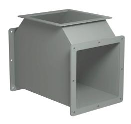
Hammond 1487 series pull-through wireway fitting, tee, 8 x 8in, carbon steel, ANSI 61 gray, powder coat finish, NEMA 12. For use with 1487 series wireway.
