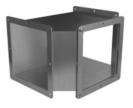
Hammond pull-through wireway fitting, tee, 8 x 8in, 304 stainless steel, #4 brush finish, NEMA 4/4X/12. For use with 1487SS series wireway.
