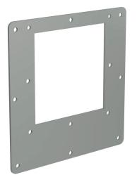
Hammond 1487 series pull-through wireway fitting, reducer, 8x 8in to 6 x 6in, carbon steel, ANSI 61 gray, powder coat finish, NEMA 12. For use with 1487 series wireway.
