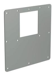
Hammond 1487 series pull-through wireway fitting, edge hole reducer, 8 x 8in to 4 x 4in, carbon steel, ANSI 61 gray, powder coat finish, NEMA 12. For use with 1487 series wireway.
