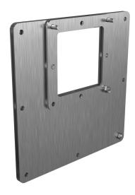
Hammond pull-through wireway fitting, reducer,  $8 \times 8$  in to  $4 \times 4$  in, edge-aligned opening, 304 stainless steel, #4 brush finish, NEMA 4/4X/12. For use with 1487SS series wireway.
