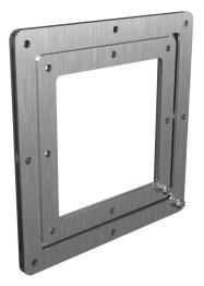
Hammond pull-through wireway fitting, reducer, 8 x 8in to 6 x 6in, center-aligned opening, 304 stainless steel, #4 brush finish, NEMA 4/4X/12. For use with 1487SS series wireway.
