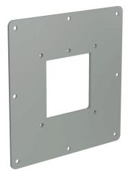
Hammond 1487 series pull-through wireway fitting, center hole reducer, 8 x 8in to 4 x 4in, carbon steel, ANSI 61 gray, powder coat finish, NEMA 12. For use with 1487 series wireway.
