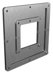
Hammond pull-through wireway fitting, reducer, 8 x 8in to 4 x 4in, center-aligned opening, 304 stainless steel, #4 brush finish, NEMA 4/4X/12. For use with 1487SS series wireway.
