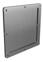
Hammond wireway fitting, cover plate, 8 x 8in, 304 stainless steel, #4 brush finish, NEMA 4/4X/12. For use with 1487SS series wireway.
