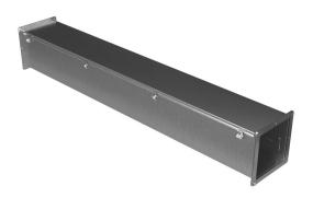
Hammond 1487SS series pull-through wireway, 8 x 8 x 60in, 304 stainless steel, #4 brush finish, screw clamps, NEMA 4/4X/12.
