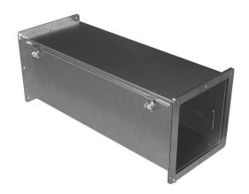
Hammond 1487SS series pull-through wireway, 8 x 8 x 24in, 304 stainless steel, #4 brush finish, screw clamps, NEMA 4/4X/12.
