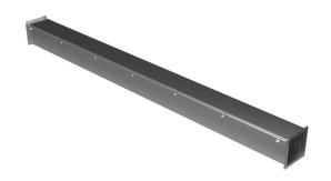
Hammond pull-through wireway, 8 x 8 x 120in, 304 stainless steel, screw clamps, NEMA 4/4X/12.
