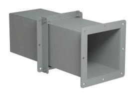
Hammond 1487 series pull-through wireway fitting, adjustable fitting, 6 x 6in, carbon steel, ANSI 61 gray, powder coat finish, NEMA 12. For use with 1487 series wireway.
