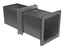
Hammond pull-through wireway fitting, adjustable fitting, 6 x 6in, 304 stainless steel, #4 brush finish, NEMA 4/4X/12. For use with 1487SS series wireway.
