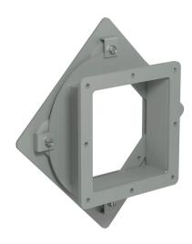
Hammond 1487 series pull-through wireway fitting, standard swivel nipple, 6 x 6in, carbon steel, ANSI 61 gray, powder coat finish, NEMA 12. For use with 1487 series wireway.
