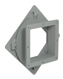
Hammond 1487 series pull-through wireway fitting, box entry swivel nipple, 6 x 6in, carbon steel, ANSI 61 gray, powder coat finish, NEMA 12. For use with 1487 series wireway.
