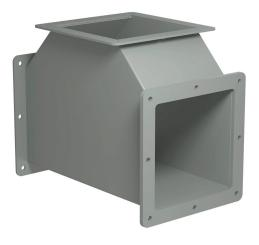
Hammond 1487 series pull-through wireway fitting, tee, 6 x 6in, carbon steel, ANSI 61 gray, powder coat finish, NEMA 12. For use with 1487 series wireway.
