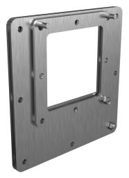
Hammond pull-through wireway fitting, reducer, 6 x 6in to 4 x 4in, edge-aligned opening, 304 stainless steel, #4 brush finish, NEMA 4/4X/12. For use with 1487SS series wireway.
