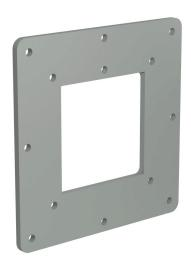
Hammond 1487 series pull-through wireway fitting, center hole reducer, 6 x 6in to 4 x 4in, carbon steel, ANSI 61 gray, powder coat finish, NEMA 12. For use with 1487 series wireway.
