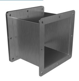
Hammond pull-through wireway fitting, nipple,  $6 \times 6 \times 6$  in, 304 stainless steel, #4 brush finish, NEMA 4/4X/12. For use with 1487SS series wireway.
