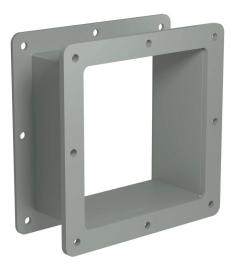
Hammond 1487 series pull-through wireway fitting, nipple,  $6 \times 6 \times 3$  in, carbon steel, ANSI 61 gray, powder coat finish, NEMA 12. For use with 1487 series wireway.
