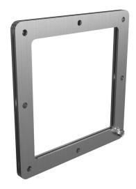
Hammond pull-through wireway fitting, box connector, 6 x 6in, 304 stainless steel, #4 brush finish, NEMA 4/4X/12. For use with 1487SS series wireway.
