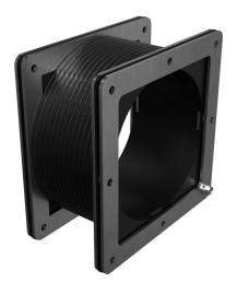
Hammond pull-through wireway fitting, flexible fitting, 6 x 6in, GortiflexTM bellows with 304 stainless steel flanges, #4 brush finish, NEMA 4/4X/12. For use with 1485 and 1487 series wireway.
