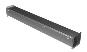
Hammond 1487SS series pull-through wireway, 6 x 6 x 60in, 304 stainless steel, #4 brush finish, screw clamps, NEMA 4/4X/12.
