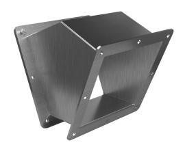
Hammond pull-through wireway fitting, 45-degree elbow, 6 x 6in, 304 stainless steel, #4 brush finish, NEMA 4/4X/12. For use with 1487SS series wireway.
