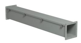
Hammond 1487 series pull-through wireway, 6 x 6 x 48in, carbon steel, ANSI 61 gray, powder coat finish, screw clamps, NEMA 12.
