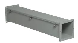
Hammond 1487 series pull-through wireway, 6 x 6 x 36in, carbon steel, ANSI 61 gray, powder coat finish, screw clamps, NEMA 12.
