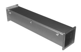
Hammond 1487SS series pull-through wireway, 6 x 6 x 36in, 304 stainless steel, #4 brush finish, screw clamps, NEMA 4/4X/12.
