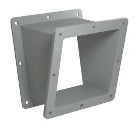
Hammond 1487 series pull-through wireway fitting, 22.5-degree elbow, 6 x 6in, carbon steel, ANSI 61 gray, powder coat finish, NEMA 12. For use with 1487 series wireway.
