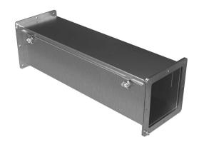
Hammond 1487SS series pull-through wireway, 6 x 6 x 24in, 304 stainless steel, #4 brush finish, screw clamps, NEMA 4/4X/12.
