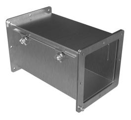
Hammond 1487SS series pull-through wireway, 6 x 6 x 12in, 304 stainless steel, #4 brush finish, screw clamps, NEMA 4/4X/12.
