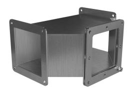
Hammond pull-through wireway fitting, tee,  $4 \times 4$ in, 304 stainless steel, #4 brush finish, NEMA 4/4X/12. For use with 1487SS series wireway.
