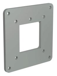
Hammond 1487 series pull-through wireway fitting, center hole reducer,  $4 \times 4$ in to 2.5 x 2.5in, carbon steel, ANSI 61 gray, powder coat finish, NEMA 12. For use with 1487 series wireway.
