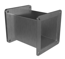
Hammond pull-through wireway fitting, nipple,  $4 \times 4 \times 6$ in, 304 stainless steel, #4 brush finish, NEMA 4/4X/12. For use with 1487SS series wireway.
