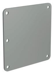
Hammond 1487 series pull-through wireway fitting, cover plate, 4 x 4in, carbon steel, ANSI 61 gray, powder coat finish, NEMA 12. For use with 1487 series wireway.
