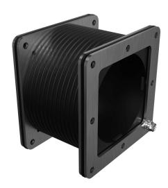
Hammond pull-through wireway fitting, flexible fitting, 4 x 4in, GortiflexTM bellows with 304 stainless steel flanges, #4 brush finish, NEMA 4/4X/12. For use with 1485 and 1487 series wireway.
