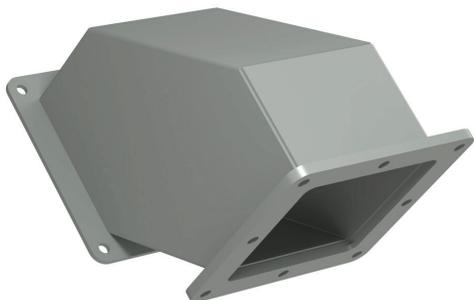
Hammond 1487 series pull-through wireway fitting, 90-degree elbow, 4 x 4in, carbon steel, ANSI 61 gray, powder coat finish, NEMA 12. For use with 1487 series wireway.
