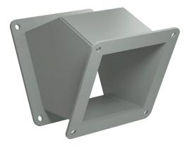
Hammond 1487 series pull-through wireway fitting, 45-degree elbow, 4 x 4in, carbon steel, ANSI 61 gray, powder coat finish, NEMA 12. For use with 1487 series wireway.
