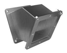
Hammond pull-through wireway fitting, 45-degree elbow, 4 x 4in, 304 stainless steel, #4 brush finish, NEMA 4/4X/12. For use with 1487SS series wireway.
