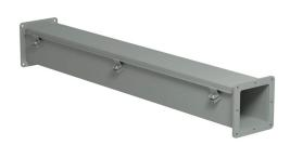
Hammond 1487 series pull-through wireway, 4 x 4 x 36in, carbon steel, ANSI 61 gray, powder coat finish, screw clamps, NEMA 12.
